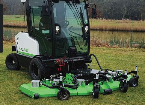
The 8015F can be equipped with **ROPS** or **cabin**.
